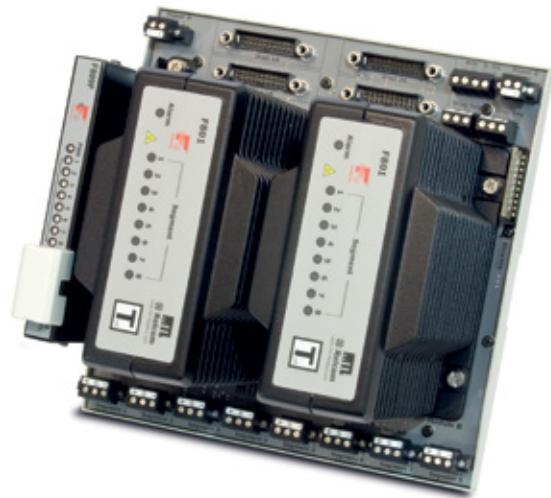
Connections to the alarm relays are made via terminals on the F882-CA-P\* carrier. A separate alarm module is not required for this function. LED indicators also show the status of each F80x module and the eight individual segments. In normal operation, each segment LED is lit, showing that the segment is powered. If a segment is shorted, this LED is extinguished, and the module Alarm LED is lit.
