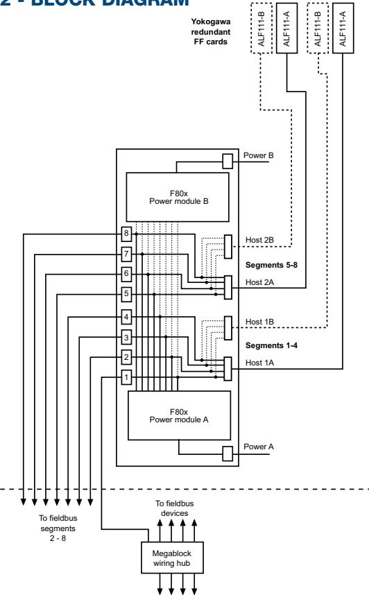
The above diagram shows a block diagram of how the F882 is wired. Note that the Chassis Ground and Alarm connection are not shown. The Diagnostic module is also not shown (see the F809F product specification). For detailed wiring information see the Installation Instructions for the F882 (Document number 502-570).
